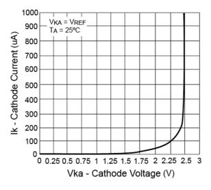
Figure 18. Cathode Current vs. Cathode Voltage
