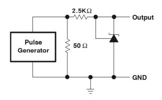
Test Circuit for Pulse Response, lk=1mA
