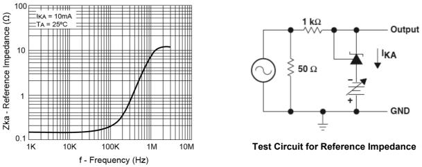
Figure 13. Reference Impedance vs. Frequency
