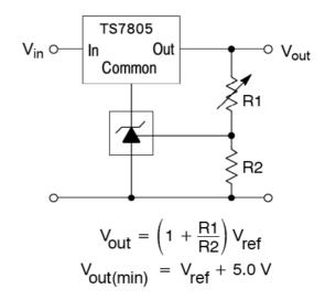
Figure 2. Output Control for Three Terminal Fixed Regulator
