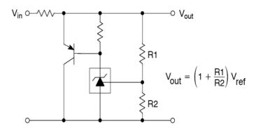
**Figure 4. High Current Shunt Regulator**
