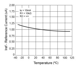
Figure 17. Reference Current vs. Temperature
