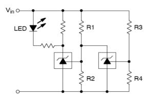
L.E.D. indicator is 'ON' when  $V_{in}$  is between the upper and lower limits,
