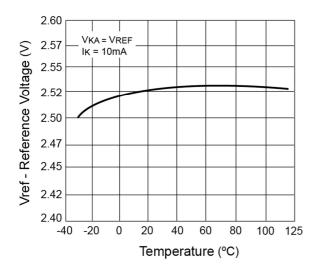
Figure 16. Reference Voltage vs. Temperature
