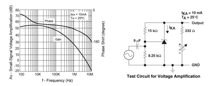
Figure 12. Small-Signal Voltage Gain and Phase Shirt vs. Frequency
