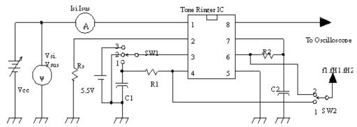
Figure 3. Test Circuit (2)
