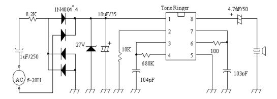
Figure 1. Ringing Start Voltage Test Circuit
