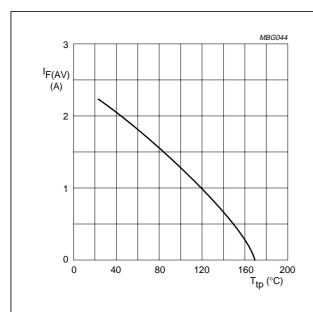
a = 1.57;  $V_R = V_{RRMmax}$ ;  $\delta$  = 0.5; lead length 10 mm.
