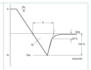
Fig. 5. Reverse recovery definitions; ramp recovery
