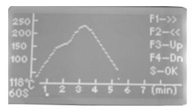
Press "F1/F2" button, forward and backward to select different time. Press F3/F4 button up and down to select different temperature, Press "s" button to save.
