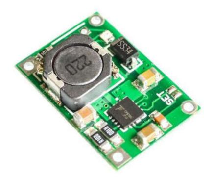
TP5100 is a double switch buck 8.4V, single cell 4. 2V lithium battery charge management chip. Its ultra-compact QFN16 package and simple external circuit, making TP5100 ideal for portable equipment so large current charging management applications. Meanwhile, TP5100 built-in input overcurrent, undervoltage protection, over temperature protection, short circuit protection, battery temperature monitoring, reverse battery protection.
