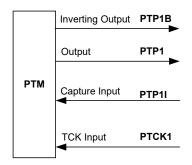
**PTM Function Pin Control Block Diagram**
