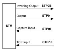
**STM Function Pin Control Block Diagram**
