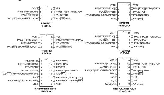
Note: 1. Bracketed pin names indicate non-default pinout remapping locations.
