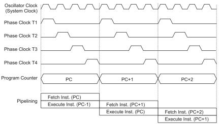
System Clock and Pipelining
