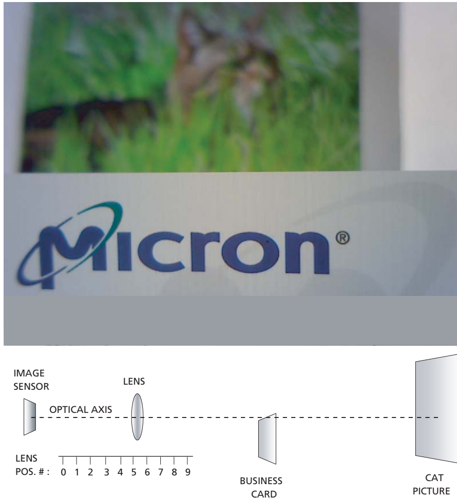
Figure 43: Scene with Two Potential Focus Targets at Different Distances from Camera
