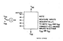
Fig. 13 - Input-current test circuit.
