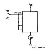
Fig. 11 - Quiescent-device current test circuit.
