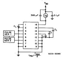
Fig. 10 - Dynamic power dissipation test circuit.
