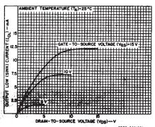
Fig. 2 - Minimum output low (sink)
