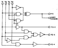
Using Couleur's Technique (BIDEC)<sup>A</sup>, a binary number (most significant bit, MSB) first is shifted and processed, such that the BCD equivalent is obtained when the last binary bit is clocked into the register. The CD4035B, with the correct conversion logic, can also be used as a BCD-to-binary converter.
