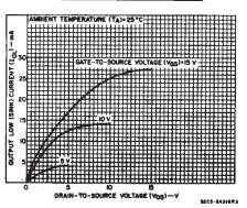
Fig. 1 — Typical output low (sink) current characteristics.
