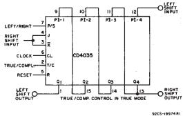
Fig. 14 — Shift left/shift right register.
