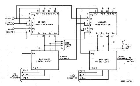
Fig. 17 - Binary-to-BCD converter.
