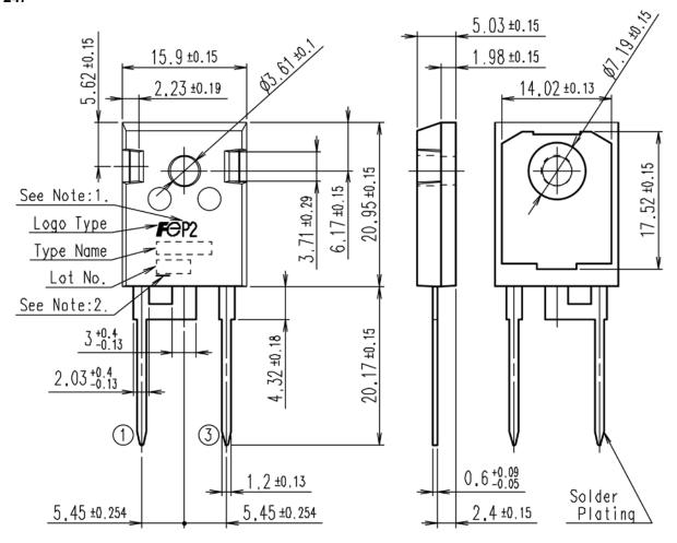
DIMENSIONS ARE IN MILLIMETERS.
