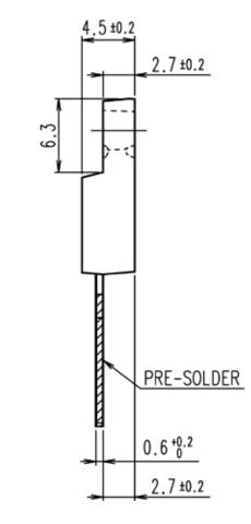
DIMENSIONS ARE IN MILLIMETERS.
