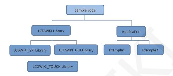
Arduino's test program code consists of two parts: the LCDWIKI library and application code.
