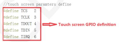
Note: The touch screen GPIO is defined using the touch test program.
