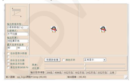
The Image2Lcd software needs to be set to horizontal, left to right, top to bottom, and low position to the front scan mode.
