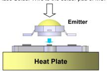
Put Emitter on MCPCB. Take the MCPCB out from Heat Plate within 10 seconds.
