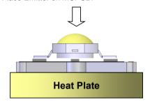
Put MCPCB on Heat Plate until Solder Paste melt. The Solder Paste sould be melted within 10 seconds. Take out MCPCB out from Heat Plate within 15 seconds.
