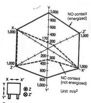
Shock directions (with coil terminals on the front side)
