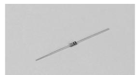
RDM is a small sized type of RD resistor and a highly reliable thermal deposition type. IT is manufactured through the rationalized automatic line and the high quality control system. Different types of the fixed carbon film resistor rating from 1/4W to 1/2W are available. They are widely used as the standard parts corresponding to automatic insertion.
