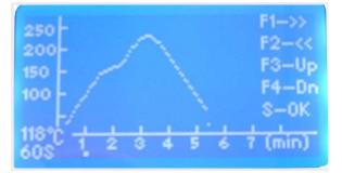
Press "F1/F2" button, forward and backward to select different time. Press F3/F4 button up and down to select different temperature, Press "s" button to save.
