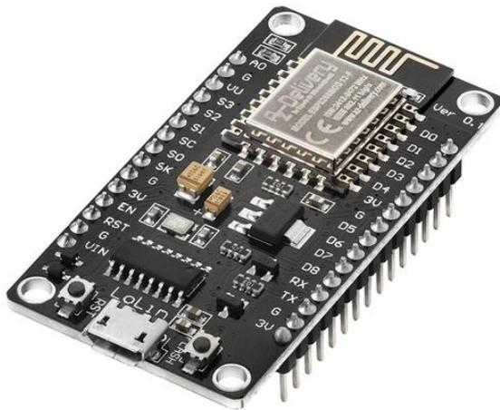
The AZ-Delivery NodeMCU Lolin V3 has many improvements compared to its predecessor. Moreover, the new USB interface provides better driver compatibility and a more comfortable transfer of firmware and code, without having to press the reset and flash buttons at the right moment. The NodeMCU is powered by a micro-USB port.
