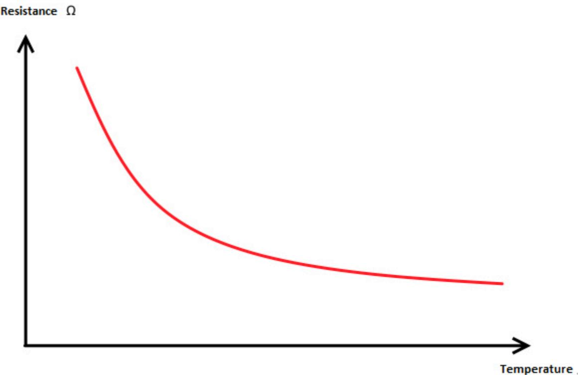
You can draw near to the resistant change via maths and convert it into a linear course. With that you can determine the temperature coefficient (addicted from resistant change to temperature change). With that you can determine the actual temperature if you know the current resistance.
