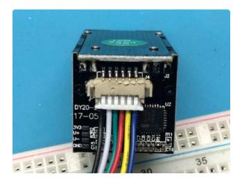
If your sensor has different wires, The first wire from the left should be the black wire ground, then the two data pins, RX is the white wire, TX is the green wire then the red power wire. You'll have to cut, strip and solder thicker gauge wires to the current wires.
