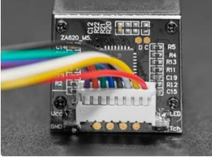
If your fingerprint sensor has individual socket wires (its this one) (http://adafru.it/ 4690) then use the following wire setup:
