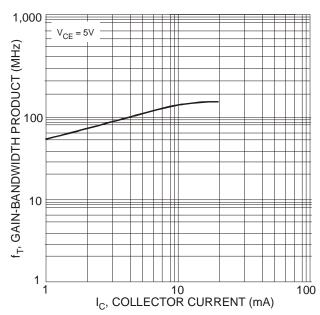
Figure 8. Typical Gain-Bandwidth Product vs. Collector Current
