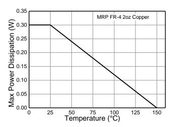
Figure 2. Derating Curve
