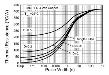
Figure 3. Transient Thermal Impedance
