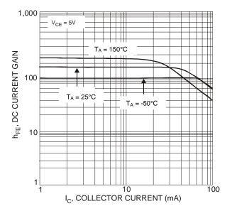
Figure 5. Typical DC Current Gain vs. Collector Current
