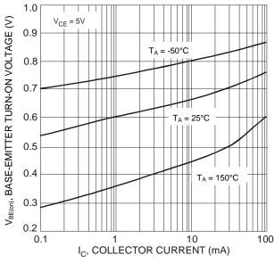
Figure 7. Typical Base-Emitter Turn-On Voltage vs. Collector Current
