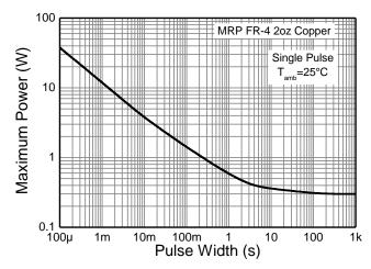
**Figure 4. Pulse Power Dissipation**
