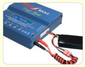
The main battery leads must be connected along with the balance lead connector as shown before charging your battery  $\dots$
