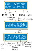
The value on the left side of the second lines sets the charge current. The value on the right side of the second lines sets the battery pack's voltage. After setting current and voltage, press STAR/ENTER formore than 3 seconds to start the process.
