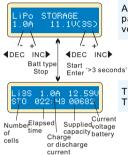
At this screen, you can set up the current and voltage of the battery pack. Charging and discharging will make the batteries come to the voltage level of "storage" state.
