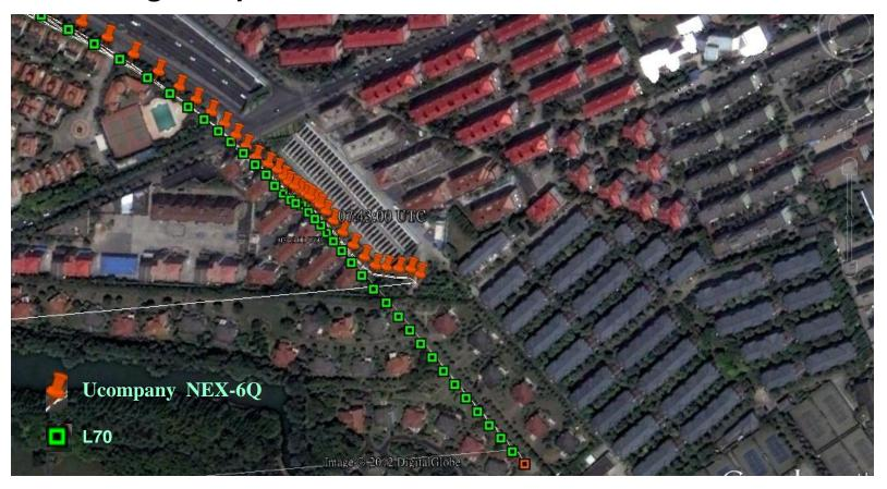
When driving into a channel, the GPS signal becomes weak. L70 can still fix position for a while.
