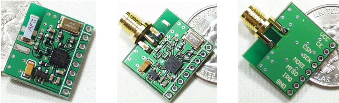
Figure 1. Left to right: MiRF-v2 top, MiRF-v2 RP-SMA top and bottom (pics from www.sparkfun.com )
