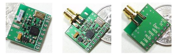
Figure 1. Left to right: MiRF-v2 top, MiRF-v2 RP-SMA top and bottom (pics from www.sparkfun.com)
