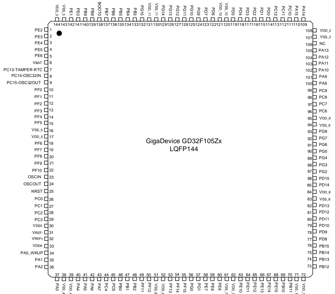
Figure 2-2. GD32F105Zx LQFP144 pinouts
