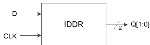
Figure 3-16 I/O Logic in DDR Input Mode
