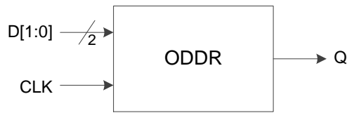
Figure 3-17 I/O Logic in DDR Output Mode
