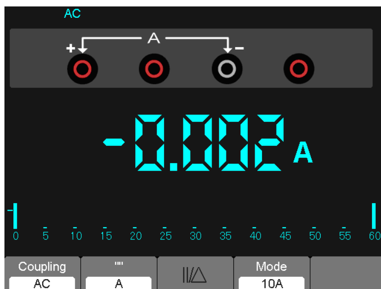
Figure 7-11 AC Current Measurement for 10A
