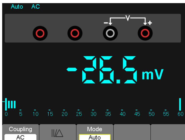
Figure 7-7 AC voltage Measurement
