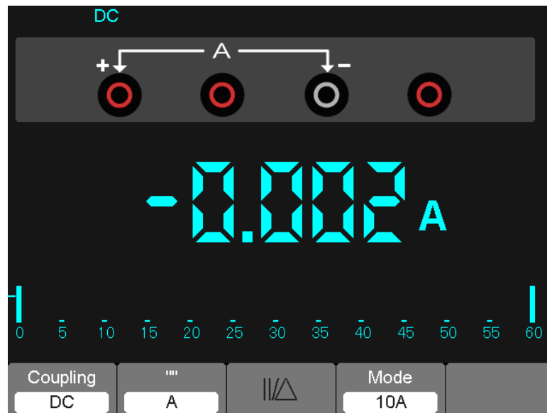
Figure 7-9 DC Current Measurement for 10A
