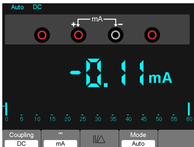
Figure 7-8 DC current Measurement for 600 Measurement
