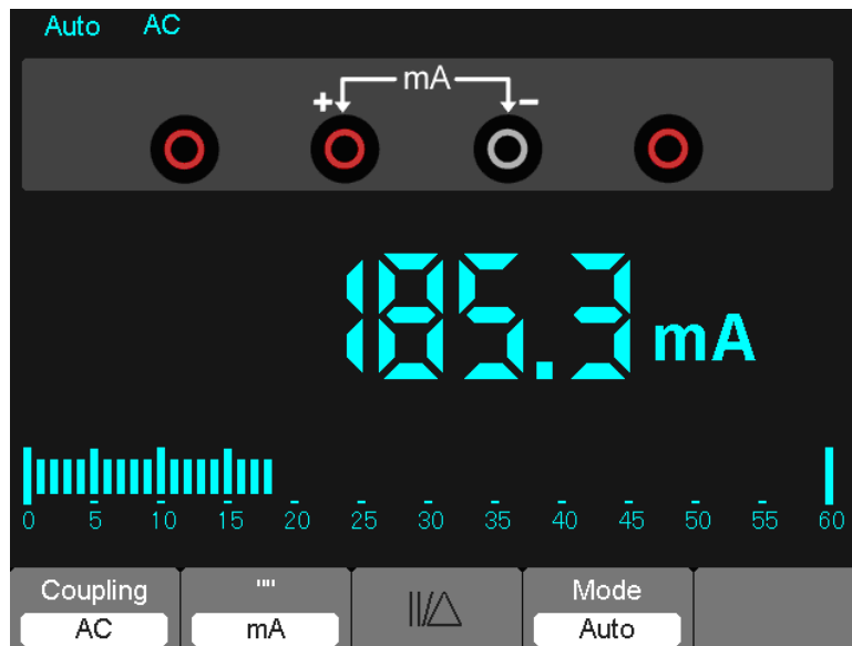
Figure 7-10 AC Current Measurement for 600 mA
