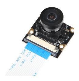
This high-quality digital camera with wide-angle lens is specially built for the Raspberry Pi and offers new possibilities. It has a 5 MegaPixel chip with a resolution of up to 2952 x 1944 Pixel. Depending on the resolution, the frame rate is up to 90 FPS. Furthermore, its application area is from 0 °C up to 50 °C possible.
