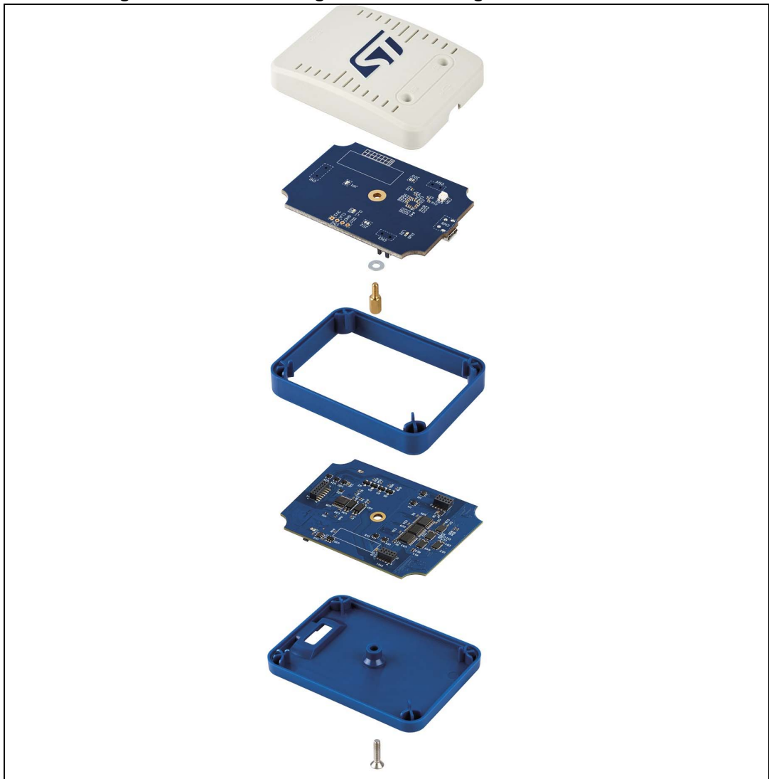
Figure 19. Closed casing for STM32 debug with B-STLINK-ISOL
