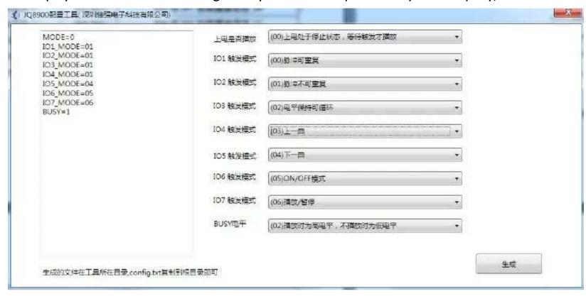
After configuring each IO port, click Generate to automatically generate a config.txt file in the directory where the software is located, and then copy the config.txt file to the memory.
