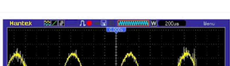
The disadvantage of only one amplitude potentiometer: it is impossible to set a small clean voltage. (© 2018 Jos Verstraten)
