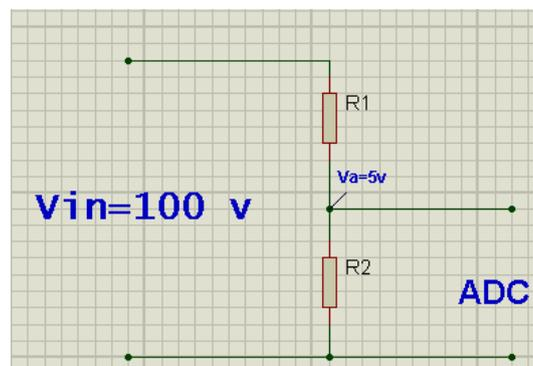
$$R_1 = \frac{R_2(V_{in} - V_a)}{V_a}$$
