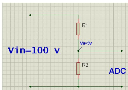
$$R_1 = \frac{R_2(V_{in} - V_a)}{V_a}$$
