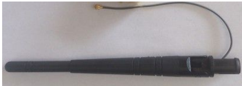
Figure 3. USR-WIFI232-T External Antenna picture
