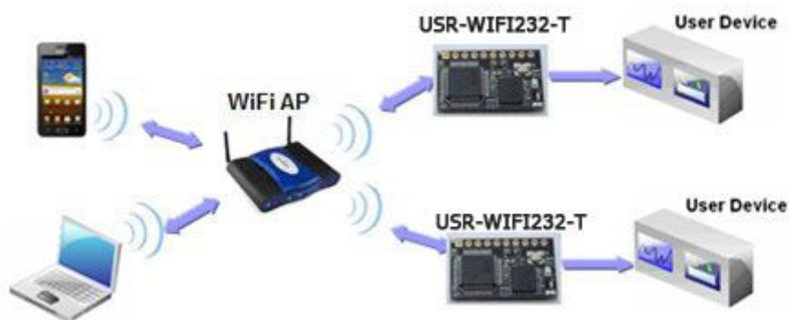
Figure 7. USR-WIFI232-T Basic Wireless Network Structure
